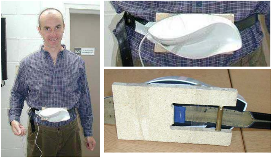
Fig. 3. Our first breath mouse, made from an optical mouse, a belt, and a piece of elastic. The mouse is fixed to a piece of wood, to which a belt is also attached. Two inches of the belt are replaced by elastic, so that changes in the waist circumference produce motion of the belt underneath the eye of the mouse. This sensor measures breathing if the user breathes using their diaphragm (rather than their rib cage). We oriented the mouse so that breathing in moves the on-screen mouse up and rotates the pointer anti-clockwise along the curve; and breathing out moves the on-screen mouse down and rotates the pointer clockwise. The sensor also responds to clenching of the stomach muscles, but we encourage the user to navigate by breathing normally.
